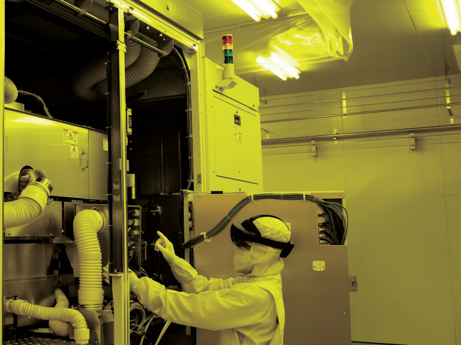
Maintenance work performed by following instructions on a hologram of a manual, viewed through a head mounted display
