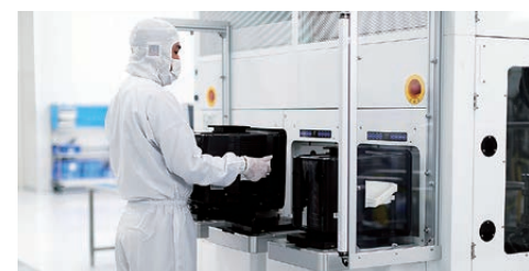
Canon ANELVA's sputtering equipment deposits uniform nanoscale film in a vacuum
