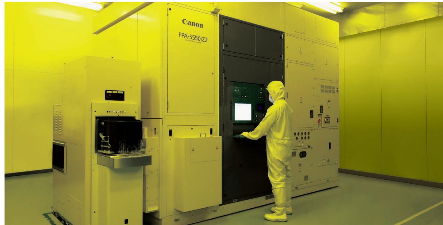
i-line stepper used to manufacture memory, image sensors and more
