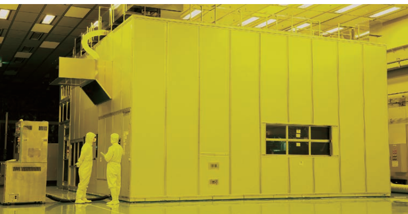
Canon FPD lithography equipment exposes circuit patterns on glass substrates
