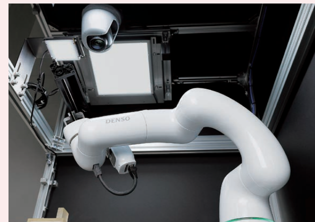
Image from network camera (top left) analyzed and orders sent to robot
